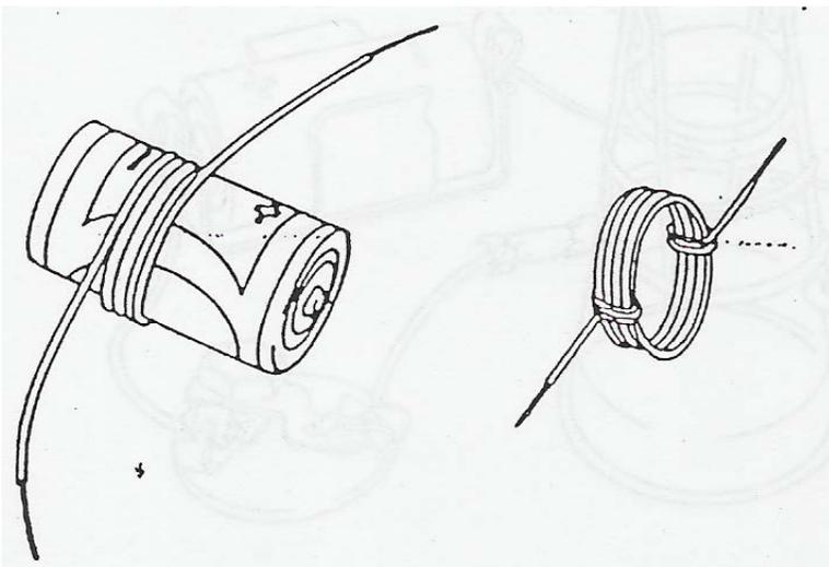
6. Next, place the ends of the coil through the loops of the bare copper wire already attached to the cup. Adjust the copper wire to fit the loop so that the loop can spin freely, without hitting anything.
