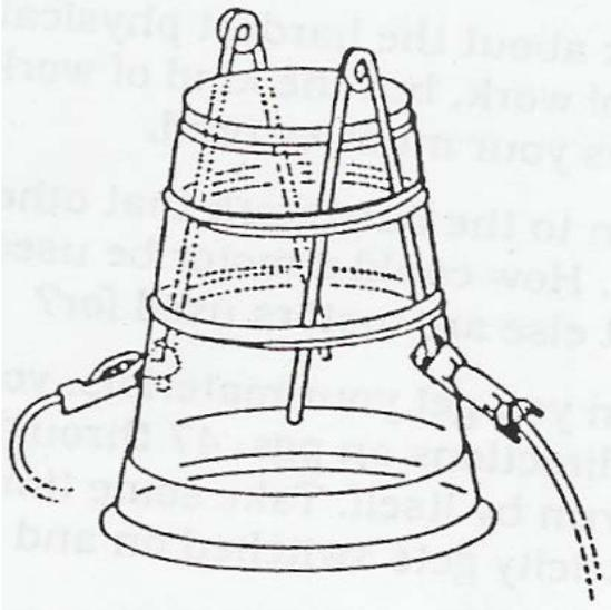
4. Next, take the longest wire with the enamel coating on it and sand off the ends so that bare wire shows through. This is so that electricity can flow from the bare copper wire through the thin wire to the other bare copper wire.
