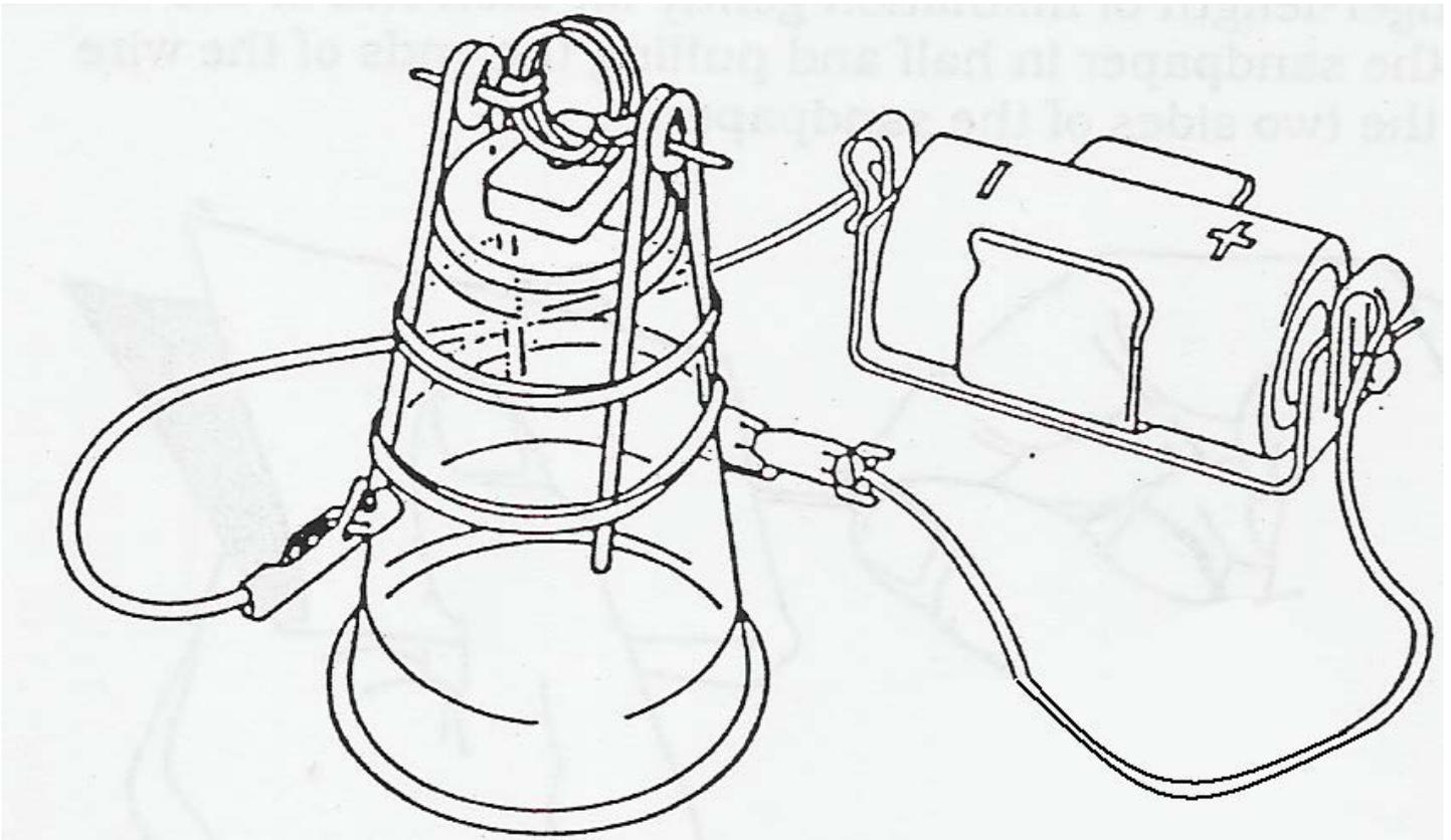
7. Place a magnet on the top of the inverted cup, underneath the coil. Touch the ends of the alligator clamps to each side of a D battery. Give the coil a slight spin to get it moving.
